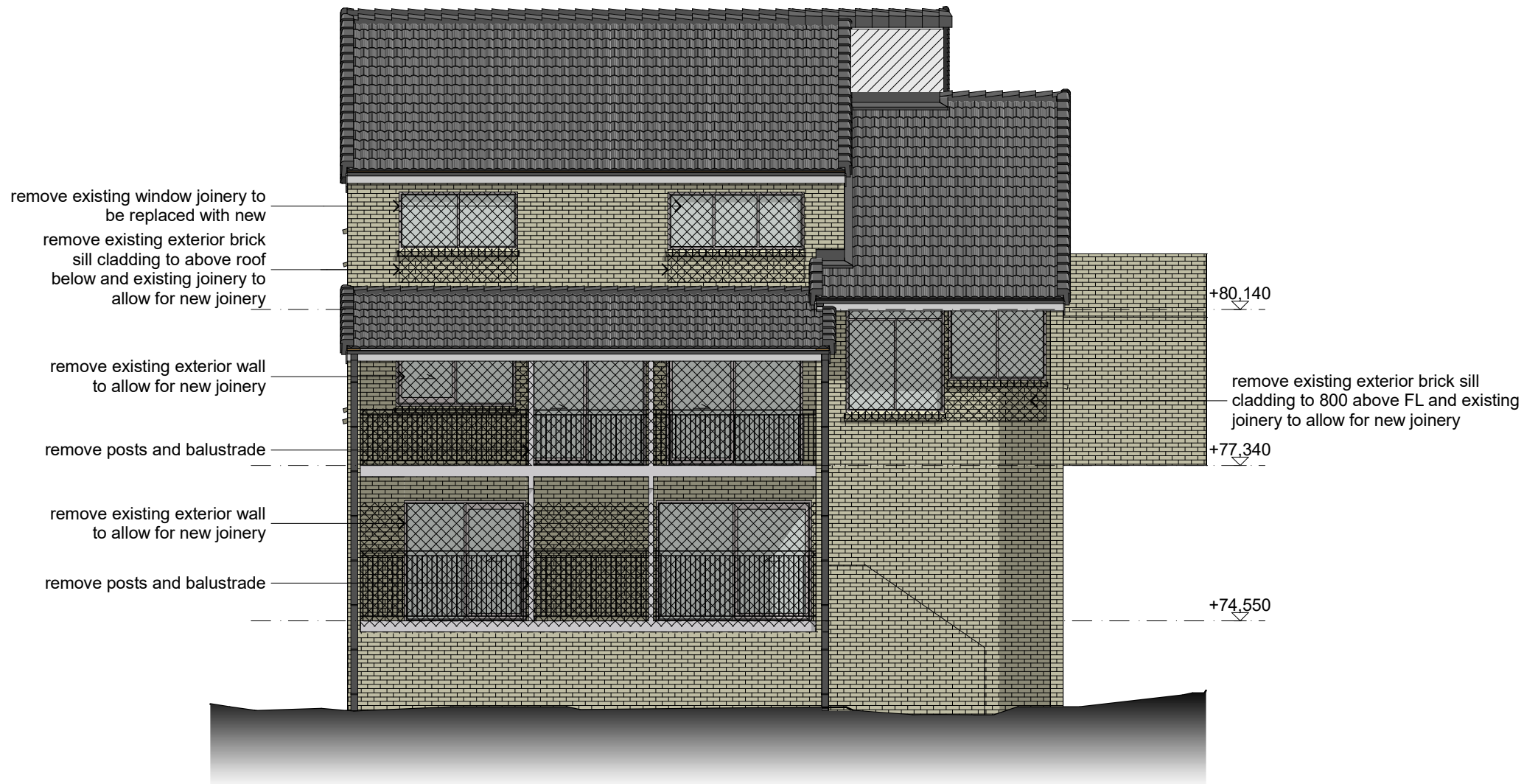
Existing/Demolition North Elevation 1:100
